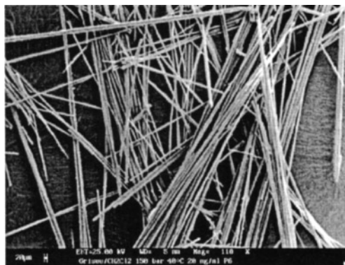
Figure 9.9-1. SEM micrographs of griseofulvin crystals precipitated from dichloromethane at 150 bar, 40°C [44].
