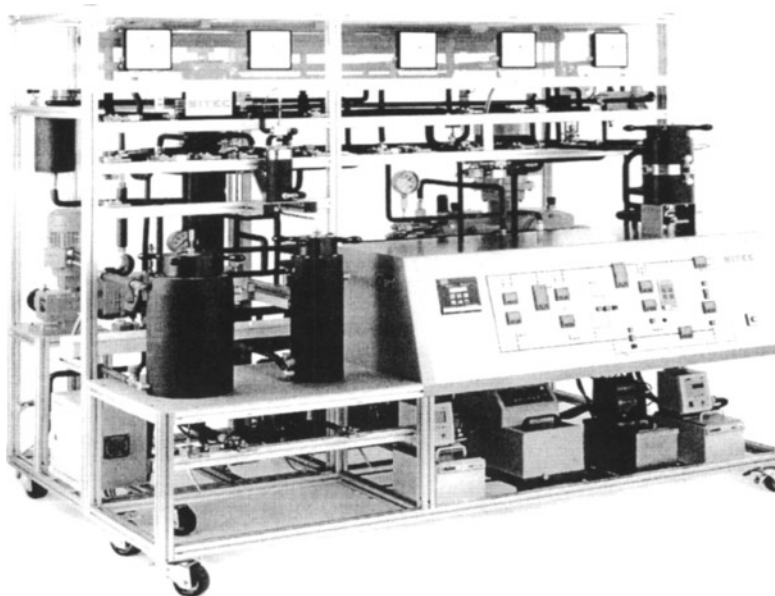
Fig. 4.3-33. SITEC super-critical fluid extraction small-scale plant [50].
